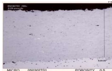
Dense RK9999 reference microstructure
